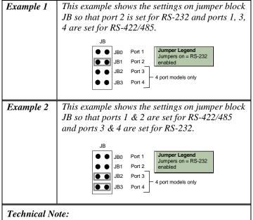
You can set up the RS-232 serial ports to run at up to 230.4 Kbps, but you must use good quality serial cables with lengths that do not exceed 2 meters.
